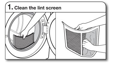
Clean the lint screen before each load. Pull the lint screen straight up. Roll lint off the screen with your fingers. Do not rinse or wash screen to remove lint. Wet lint is hard to remove. Push the lint screen firmly back into place. For additional cleaning information, see "Dryer Care."
