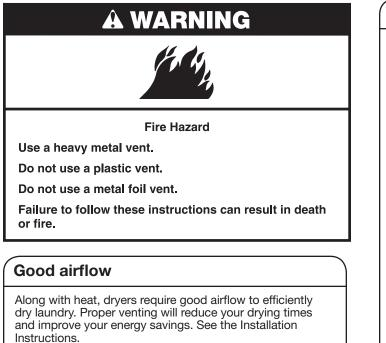
The venting system attached to the dryer plays a big role in good airflow. Blocked or crushed vents as well as improper venting installation will reduce airflow and dryer performance.
