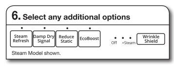
Add additional options such as Reduce Static, Wrinkle Shield, and/or EcoBoost (on some models) by touching that option. If you will be unable to remove the load promptly, select Wrinkle Shield before touching START/PAUSE. You may select the "+ Steam" setting (on some models) to add a short steam cycle after 60 minutes to help smooth out wrinkles.
