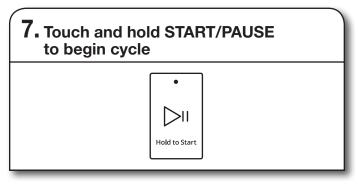
To begin the cycle, touch and hold START/PAUSE until the display counts down "3-2-1" and the dryer starts.
